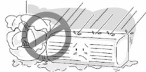
**2. Do not install in a place where flammable gas may leak .**
