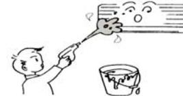
Splashing water on the air conditioner can cause an electrical shock and malfunction on the unit.
