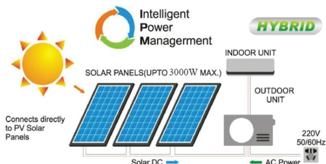
**Advantage of Solar Hybrid Air Inverter**
